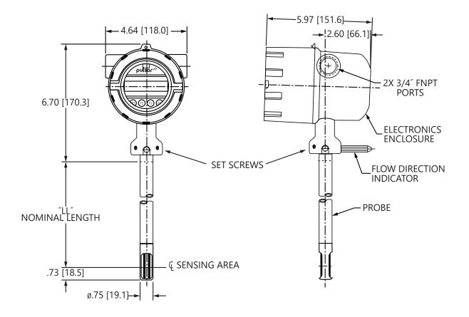
Table 7.2 Insertion Meter with 316 stainless steel probe
