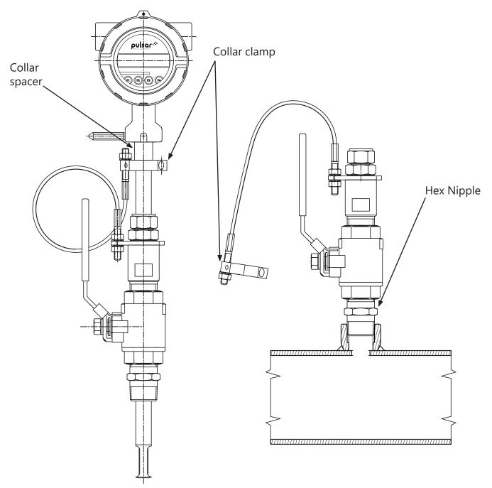
4. Carefully slide the probe through the retractor assembly and through the hole to see if there is interference by touching the pipe wall with the end of the probe on the far side or until the probe cannot go deeper. Remove the probe. Remove the retractor and rework the hole, if required.
