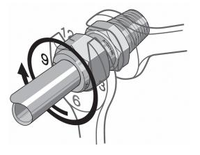
**CAUTION!** For a 1<sup>1</sup>/<sub>2</sub>" pipe, do not tighten compression fitting without 0.2" distance from wall or damage to probe will occur.
