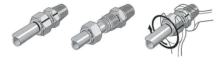
**CAUTION!** Do not use a gap inspection gauge with reassembled fittings.
