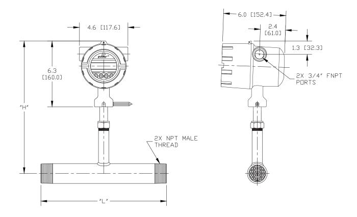
Fig. 7.3 Inline Meter with 316 Stainless Steel Flow Body and NPT End Connections Dimensions
