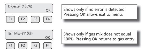
**NOTE:** The gas selection must be valid or the Digester gas mix must have a valid 100% mixture before the user is allowed to exit.
