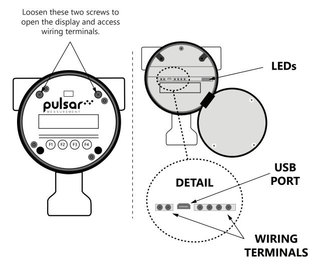
To wire the MDot, unscrew and remove the enclosure cap. If the meter has the display option, loosen the two captive screws on the display assembly and rotate it open to access the wiring terminals. Connect the power and signal wires to the terminal blocks according to the label and instructions on the following pages.
