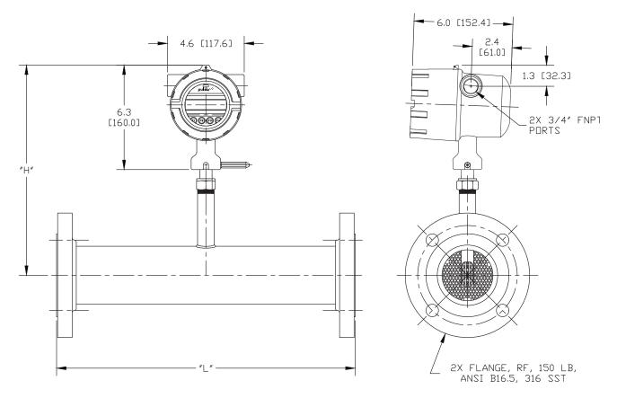
Table 7.4 Inline Meter with Choice of Flow Body and 150lb RF Flange End Connections Dimensions
