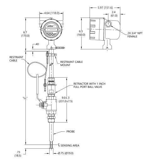
Table 7.1 Insertion Meter with 316 stainless steel probe
