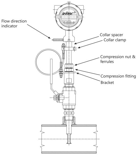
**NOTE:** For instructions on how to properly remove and replace the meter from a retractor, please refer to "Instructions for Removing and Inserting the Meter from a Pressurized Pipe using the Retractor" on page 85.
