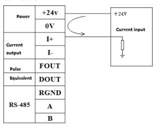
2) Three-wire system current connection method:
