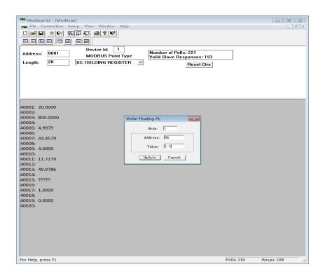
Flow coefficient communication modification method (Command No. 10 (send in HEX format)):
