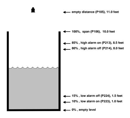
In this example, when the level rises to 8.5 feet relay 1 will come on until the level drops to 8.0 feet when it will turn off. If the level drops to 1.0 feet, then relay 2 will come on until it rises 1.5 feet when it will turn off.
