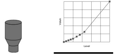
You should enter a level/volume breakpoint for each place where the vessel changes direction, and several where the section is slightly curved (mostly linear but has got a small arc). You can enter any number of pairs between 2 and 32...
