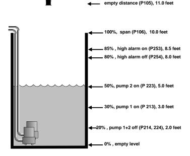
In this example, there are two pumps, which will be set to **alternate duty assist**, so they come on alternately. Pump 1 is to be set to relay 1, pump 2 to relay 2, and the high-level alarm to relay 5.
