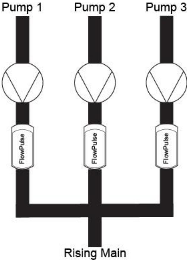
In configuration 2 each of the FlowPulse will be allocated to the pumps they are attached to. Without a FlowPulse allocated to 'All' the summation of flow being measured by all FlowPulse will be used to totalise and output flow.
