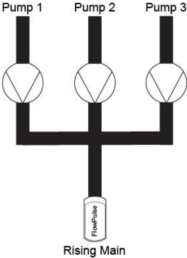
In configuration 1 the FlowPulse attached to the 'Rising Main' should be allocated as an 'All' FlowPulse (P1131, P1151, P1171, P1191). This will ensure that this FlowPulse is the only one used to totalise and output flow.
