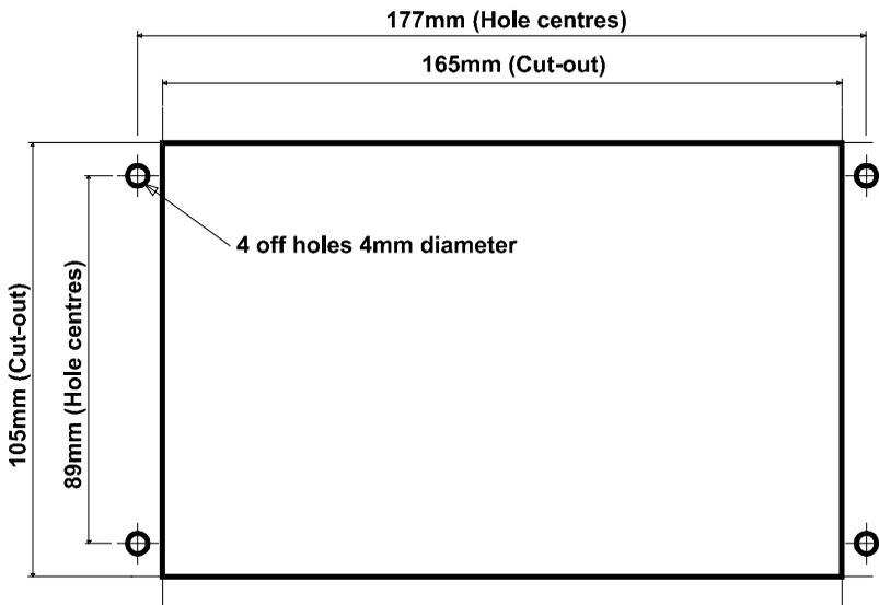
The full dimensions of the enclosure are as shown below.
