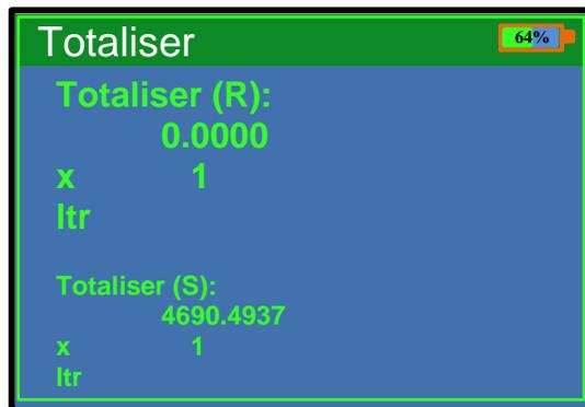
This window displays the current value of the resettable and system totaliser. The totaliser will appear during Run mode when the totaliser screen is selected. Pressing the left-hand arrow key from the Flow window will display the Totaliser window.
