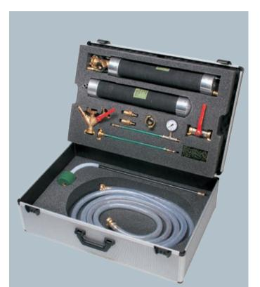
This set is used for DN 100 to 200 mm pipe leak tests using air or water as the testing medium. They can be used both in straight sections of the pipe and in section with round or sharp bends. The set consists all the necessary fittings and accessories for carrying out leak tests according to DIN EN 1610.
