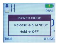
Stand-by mode is intended to be used to put the meter in a low-power state, while keeping the processor awake so that periodic data logs can be made by returning to normal-power, taking the measurement, then returning to low-power standby again. This "standby logging" functionality will form part of a later release, therefore it is not recommended that the meter is placed into standby mode since the battery will drain significantly faster than if completely off.
