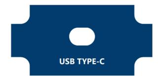
USB-C is a USB connector system with a rotationally symmetrical connector. Devices connected to USB-C may be hosts or peripherals. The PTFM 6.1 is able to make itself both, referred to as "Dual-Role-Data (DRD)" or "USB On-The-Go".
