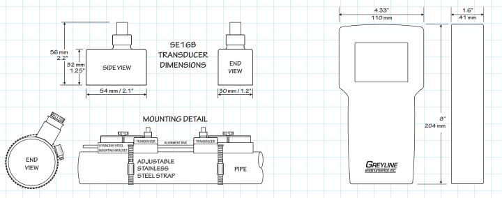
Non-Contacting Portable Flowmeter for Clean Liquids in Metal
