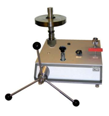
High-pressure Deadweight Tester/Pressure Balance CPB5000-HP
