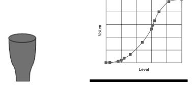
You should enter 2 level/volume breakpoints at the minimum and maximum levels, and several for each place where the vessel has got an arc. You can enter any number of pairs between 2 and 32.
