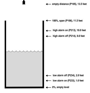
In this example, if the level rises to 10.0 feet, then the high-level alarm (relay 1) will come on until the level drops to 9.0 feet. If the level falls to 1.0 feet, then the low-level alarm (relay 2) will come on until the level rises to 2.0 feet.
