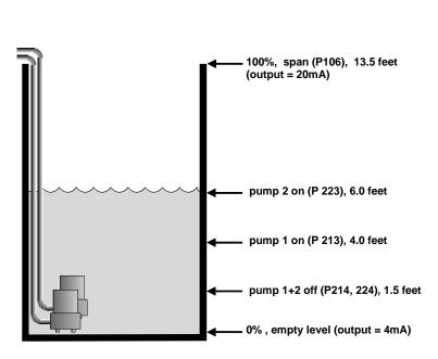
In this example a blackbox with dB6 is being used to control pumps on a **pump down** application, there are two pumps, and the **duty** pump is to be **alternated** between the pumps.
