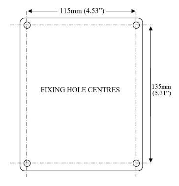
The blackbox should be mounted by drilling four holes suitable for size 8 pan or round headed screws. The screw length will be dependent on the wall to which the blackbox is to be mounted to, if it is unclad use 1.5" long screws with suitable wall fixings, if the wall is clad add the cladding thickness to the 1.5" screw length.
