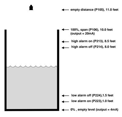
In this example, the blackbox and dB6 is being used to monitor a moving level within a vessel and is required to provide a 4 to 20mA output proportional to the level, over a range of 10.0 feet. In addition, when the level rises to 8.5 feet, Relay '1' is required to give a high alarm and rest when the level falls to 8.0 feet. In the event that the level should fall to 1.0 feet then Relay '2' is to give a low alarm and reset once the level rises to 1.5 feet.
