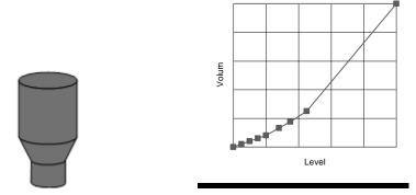
You should enter a level/volume breakpoint for each place where the vessel changes direction, and numerous where the section is slightly curved (mostly linear but has got a small arc). You can enter any number of pairs between 2 and 32.
