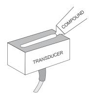
Use the pipe clamp and rail (supplied) as illustrated above or use a loop of electrical tape for temporary mounting. Apply silicon coupling compound #4 to the colored face of the transducer. A bead, similar to toothpaste on a toothbrush, is ideal. Do not overtighten (crush the transducer).
