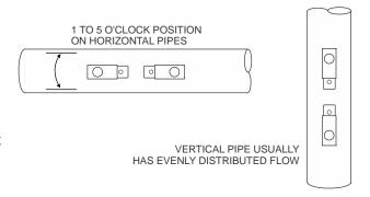
VELOCITY INCREASING DEVICES: Generally the transducers must be mounted away from flow disturbances such as valves, pumps, orifice plates, venturis or pipe inlets and discharges which tend to increase flow velocity. Velocity increasing devices often cause cavitation, or rapid release of gas bubbles, and readings both up and downstream may be intermittent or inaccurate. As a guideline, mount the transducer at least 20 diameters upstream or 30 diameters downstream from velocity increasing devices.
