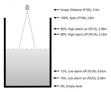
In this example, when the level rises to 2.38 m, relay 1 will come on until the level drops to 2.24 m when it will turn off. If the level drops to 0.28 m, then relay 2 will come on until it rises 0.42 m when it will turn off.
