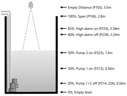
In this example, there are two pumps, which will be set to **alternate duty assist**, so they come on alternately. Pump 1 is to be set to relay 1, pump 2 to relay 2, and the high-level alarm to relay 3.
