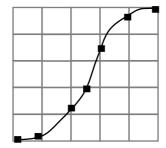
You should enter 2 level/volume breakpoints at the minimum and maximum levels, and several for each place where the vessel has got an arc. You can enter any number of pairs between 2 and 32.
