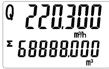
Figure 3-2 Instant flow rate and totalized flow value
