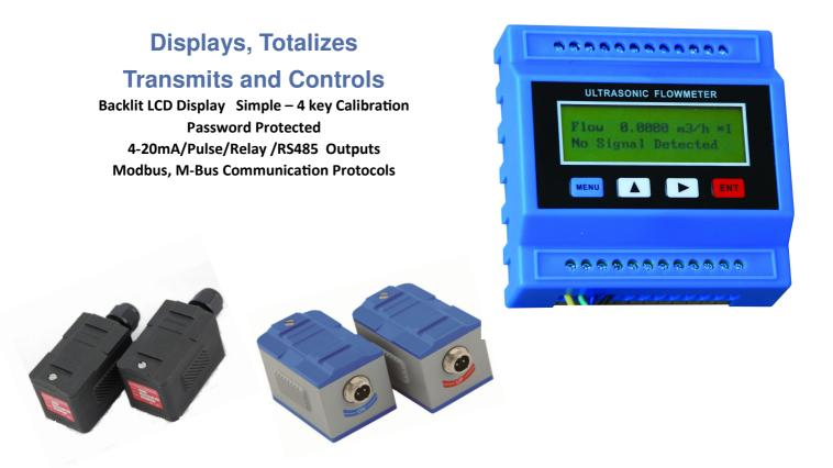
Non-Contacting Flow Measurement Ultrasonic transducers mount on the outside of plastic or metal pipes to measure flow rate of clean, non-aerated fluids like water, chemicals, and oils. The clamp on transducers can be mounted without shutting down flow. There is no pressure drop and no obstruction. Transducer separation distance is calculated by the flowmeter according to pipe diameter and wall thickness.
