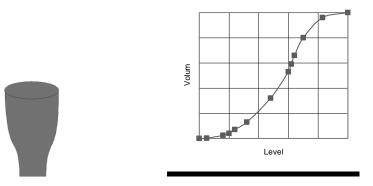
You should enter 2 level/volume breakpoints at the minimum and maximum levels, and several for each place where the vessel has got an arc. You can enter any number of pairs between 2 and 32.
