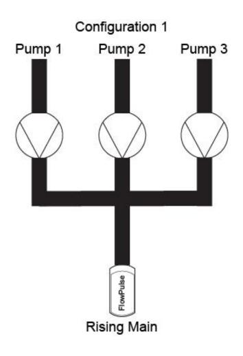
In configuration 1 the FlowPulse attacked to the 'Rising Main' should be allocated as an 'All' FlowPulse (P1131, P1151, P1171, P1191). This will ensure that this FlowPulse is the only one used to totalise and output flow.
