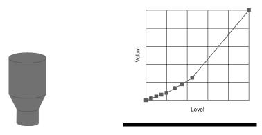
You should enter a level/volume breakpoint for each place where the vessel changes direction, and numerous where the section is slightly curved (mostly linear, but has got a small arc). You can enter any number of pairs between 2 and 32.
