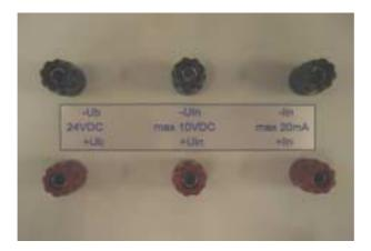
The electrical connection of a test specimen (pressure transmitter) is based on the following table:
