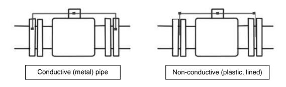
Sensor grounding with earthing rings:
