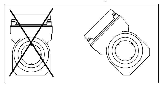
In this position, if there are any air bubbles or if sediments accumulate in the lower part of the flowmeter, it will could have an adverse effect on the earthing, which could influence the accuracy of the measurement.
