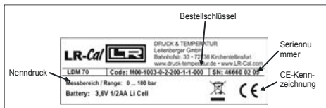
Fig. 1 manufacturing label (Nenndruck = nominal pressure; Bestellschlüsse = order code; Seriennummer = serial number; CE-Kennzeichnung = CE mark)
