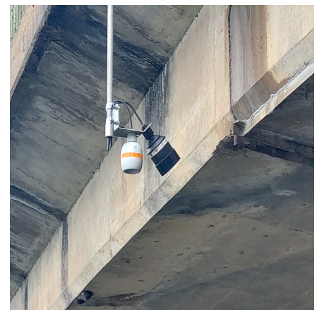
FarSight™ and REFLECT™ mounted with dBA0008 angled mounting bracket for area-velocity flow measurement
