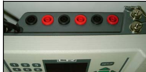
LPC 300 electr. measurement plugs voltage & current input, voltage output, pressure switch, USB/RS232, battery charger
